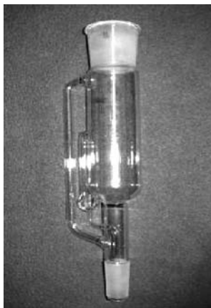
Figure 20.3. Soxhlet Extractor Glassware
